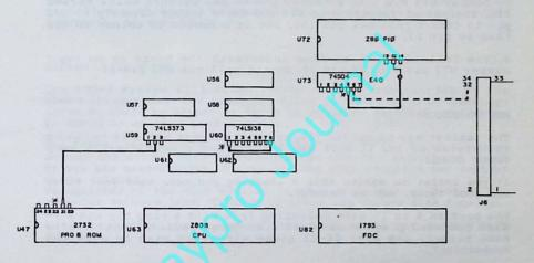
BE SURE THE PINS MARKED WITH ASTERISKS ARE PULLED OUT OF THEIR SOCKETS (Remove the chip; bend out the pin just enough so it won't go back into the socket, and then reinsert the chip. But be careful, if you bend the pin too much you might break it off.). (William Fankboner did the original parts layout diagram that we worked from. Thanks, Bill.)
