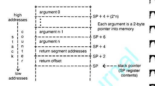
Figure 6.1. Stack layout when CALL statement is activated
