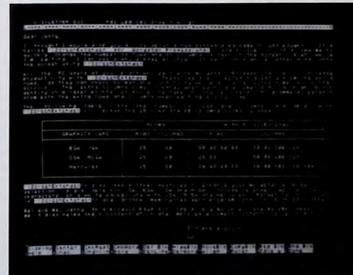
50 rows by 91 columns. Actual photo of EGA display.
